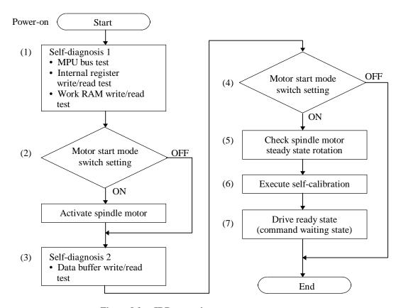
Figure 8.2 IDD operation sequence at power-on
